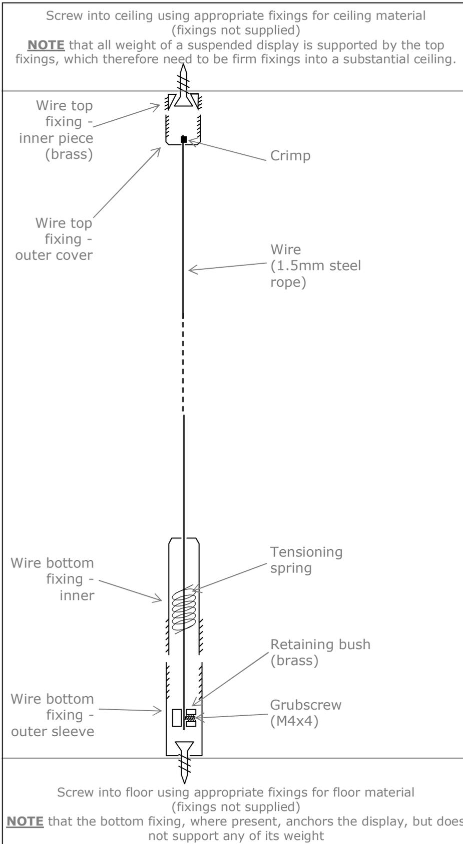
1. Mark the required positions of the wire top fixings on the ceiling.
