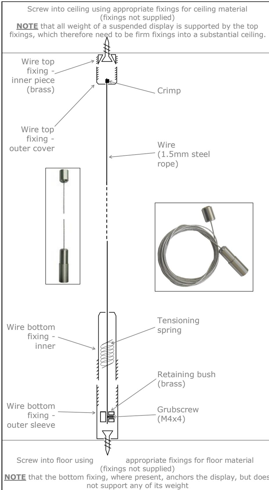
1. Mark the required positions of the wire top fixings on the ceiling. The table on page 3 shows the wire centres required for the different standard sizes of poster holders.
