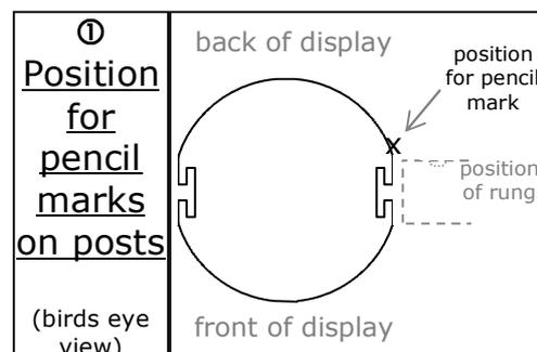
4. Tighten locks to fix rungs securely into second post, adjusting position as necessary so that rungs line up with pencil marks.
